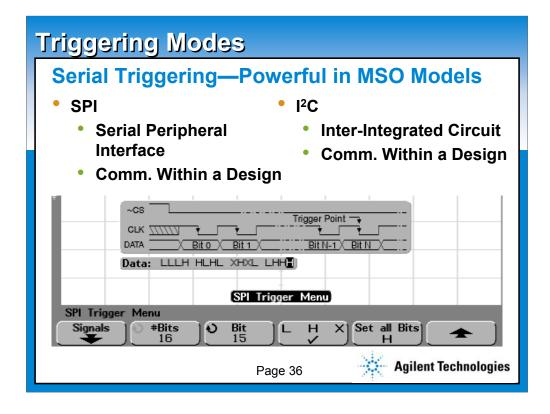
Serial communication is becoming more and more of a common place in a wide variety of applications. Remember in the example circuit of an electric meter how many different signals types were present, including analog, parallel, and serial. The fact that serial communication is present in many mixed-signal designs makes serial triggering especially important in Agilent's MSO products. Thus, the 54600-series products contain widely used protocol-specific serial triggering capabilities.
