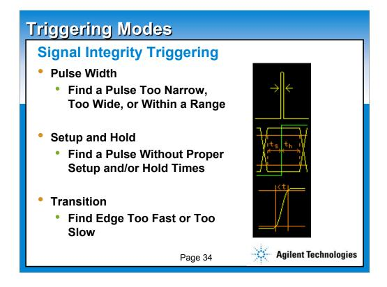
Signal Integrity triggering is important in digital design applications. It is a type of triggering in which the oscilloscope will find a point in the signal that violates certain condition(s) specified by the user. Three types of signal integrity triggering are Pulse Width, Setup and Hold, and Transition.
