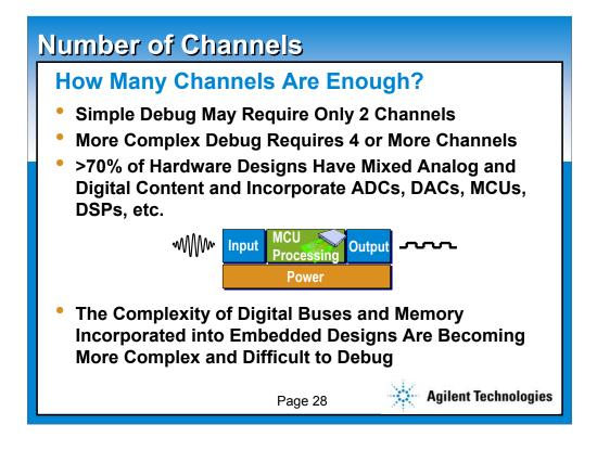
When selecting an oscilloscope, one of the basic selection criteria is determining how many channels are enough. Oscilloscopes are often times used in a multitude of applications at a single site. So often times, one would consider their most demanding application to determine how many channels are enough for selecting the right oscilloscope. Simple debug applications may require only 2 channels. More complex debug may require 4 channels...or even more!
